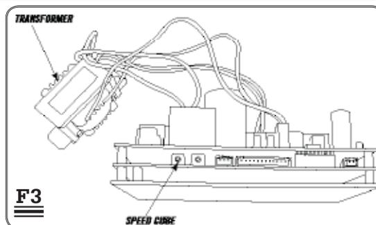
**Tip:** Another way to verify the speed is set correctly: Count the running belt revolutions per minute. At 0.5mph the running belt should make 4 revolutions per minute for the Alpine and Advance 500 and 4.5 revolutions per minute for all other units.
