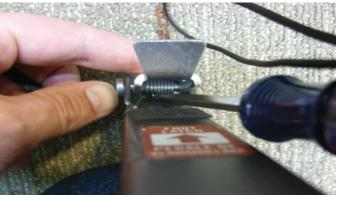
9) Reverse Steps 1-4 to re-assemble the treadmill. *NOTE:* Make sure that the lock latch is depressed and soundly in the hole in the chrome tube before tipping the treadmill upright.
