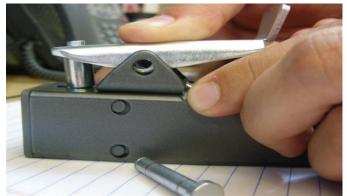
8) With the lock latch / spring pressed into place on the frame tube, insert the pin to hold the lock latch / spring to the frame tube. *NOTE:* You may need to pry up one side of the spring / pin with a flat screwdriver so that the pin will go through both sides of the frame tube.
