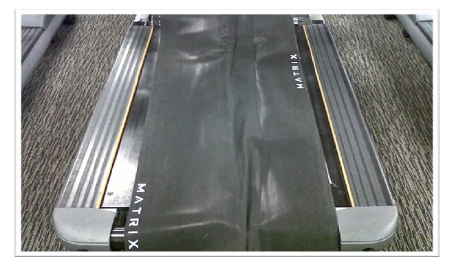
We need to be careful and inspect the running belt when you have an issue like this, it could be that the running deck is cracked and causing this issue. If you attempt to loosen the running belt and reposition the belt to its normal state, the belt will buckle again since the threads in the underside of the belt are not strong enough anymore.
